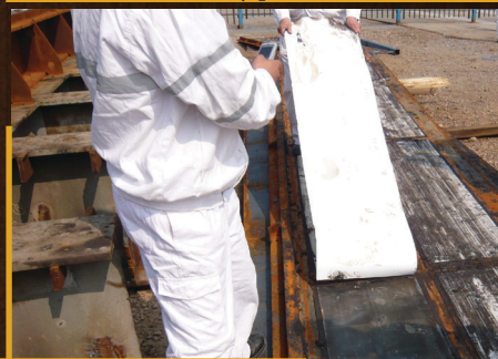
The failure of PTFE skidway plate, manufactured by a local yard with poor materials and technology
